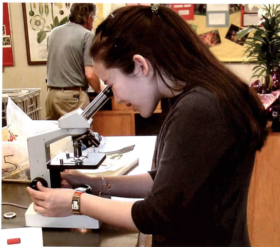
Figure 11.1 This student is using the fine adjustment knobs to focus on a microbe under high magnification.
