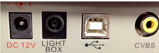
3. Make sure the power cable is also plugged into the document camera. In the photo above it is the round port on the left. It will normally be labeled with DV and a number of volts.
